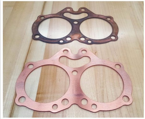
Copper gasket, precisely traced and cut to match original.
